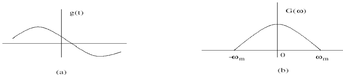
Figure 2: (a) Original signal g(t) (b) Spectrum G(\omega)
